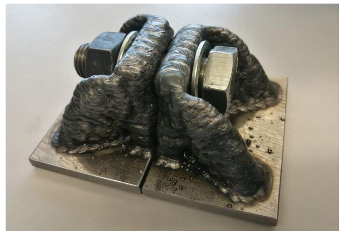
Figure 16 Final printed and connected structure
