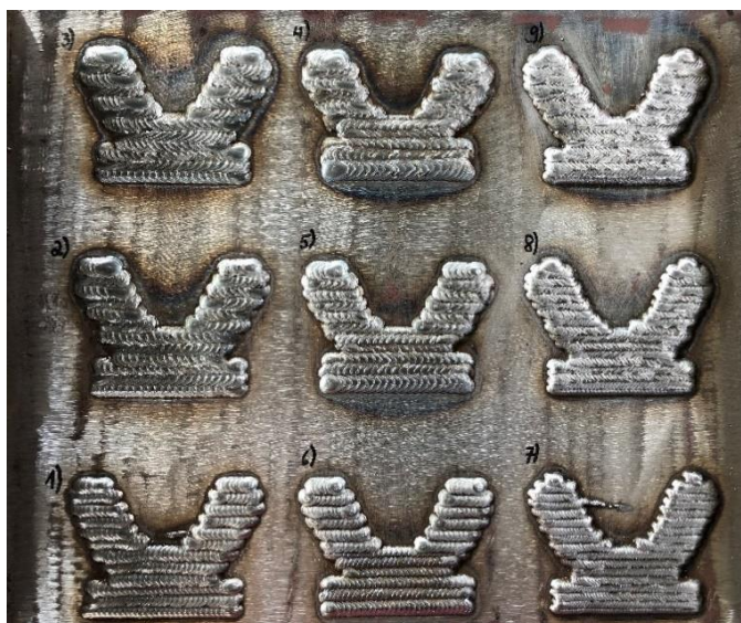
Figure 10 First printed layer of the parameter study
