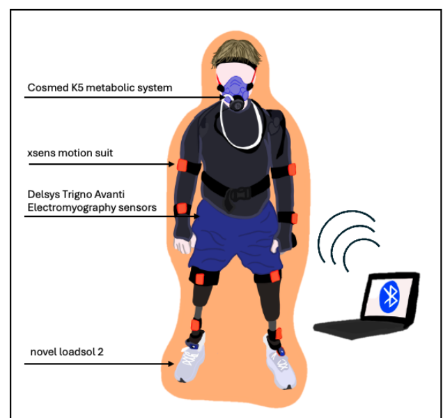
Figure 1: Schematic of the portable measurement equipment used.
