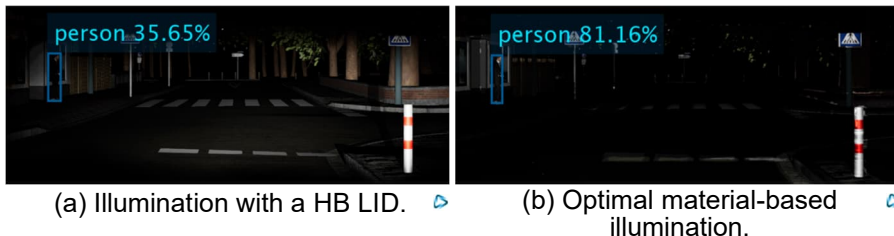
Figure 1: Confidence and BBoxes of a neural network-based detection for a pedestrian with different LIDs in the simulation [1].
