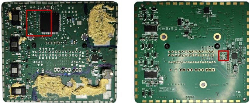
Figure 6: Comparison of a conventional light control unit with MCU (100-pin, left) and an SDV-optimised control unit with endpoint (32-pin, right).
