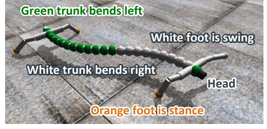
Figure 3: Simulation shows trunk flexion (green/white) and foot ground contact phases (orange/white).
