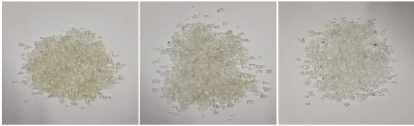
Figure 2: PC PCR from shredded headlight covers (from left to right: Group I, Group II and Group III).
