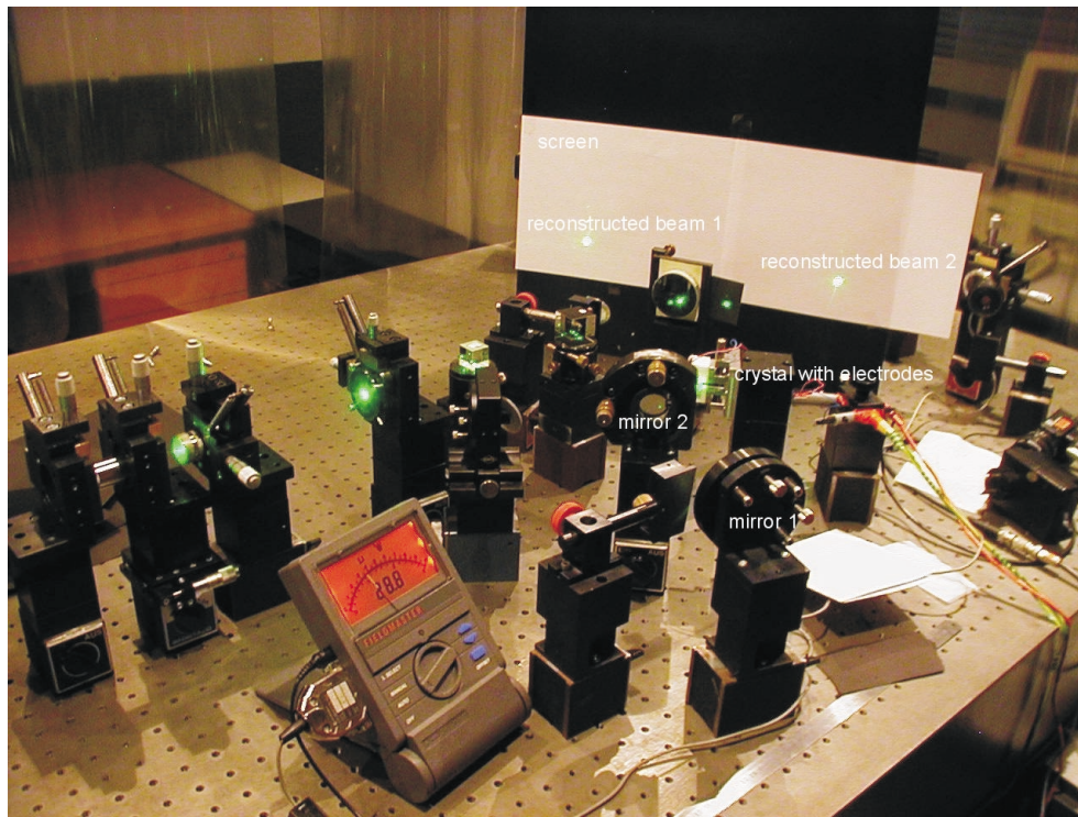
Figure 4.21: Picture showing the experimental set-up and the location of the reconstructed beams with a field of 1 kV/cm applied to the crystal (both the holograms are reconstructed).
