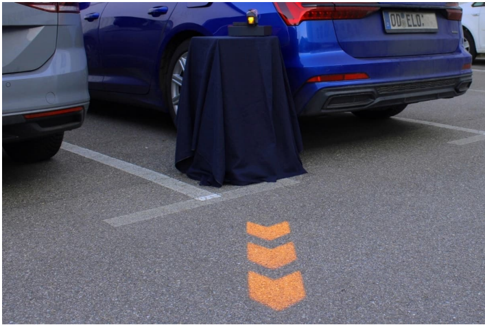
Figure 8: Photo of the signal road projection in the odelo parking lot in the shade on a sunny winter day. This photo was taken at 4 p.m. on February 3, 2025. No adjustments or manipulations have been applied to the photo, except for obscuring the license plate.
