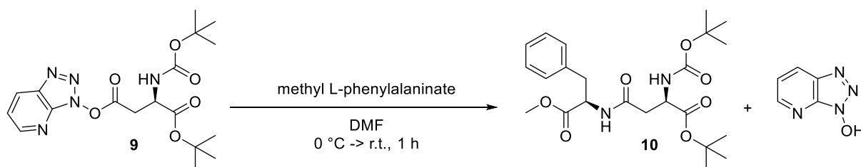
Figure 41: Coupling of the active-ester with methyl L-phenylalaninate.
