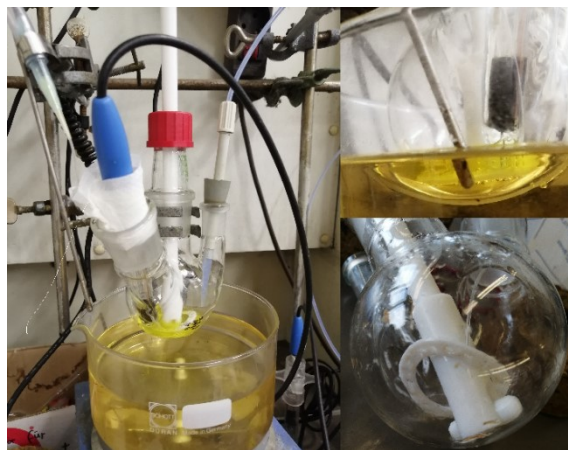
Figure 66: Teflon scaffold with interwoven silicon tube as employed in early cascade reactions. During the reaction (top right) gas bubbles visibly formed, stationary on the surface of the tube.
