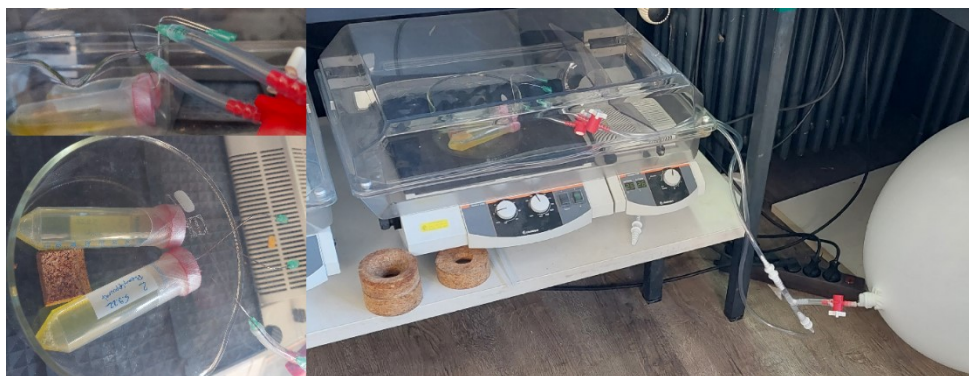
Figure 68: Facile and effective oxygen supply to cascade reactions at 20 mL-scale.
