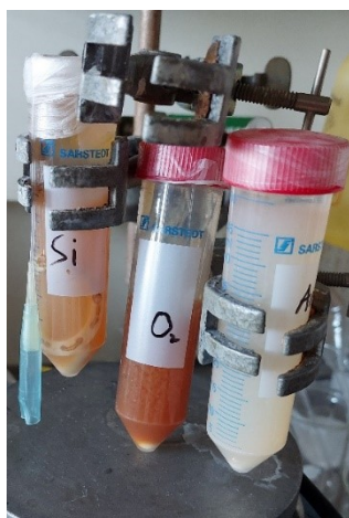
Figure 62: Visible difference in the amount of formed \text{MnO}_2 during the modified Winkler protocol. One tube was stirred and bubbled with oxygen ( \text{O}_2 ), one was stirred, while a semipermeable silicon membrane, internally pressurized with 2 bar of oxygen, was submerged (Si) and the third one was stirred while sealed.
