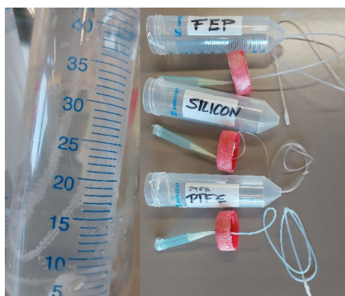
Figure 63: Setup of the oxygen dissolution tests with stationary gas bubbles visibly formed on the submerged tube (left).
