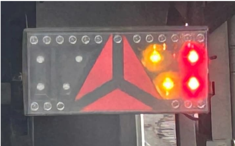
Picture 1: Rear light of a truck trailer with unnecessarily high luminance. The visibility is based on glare effects in the eye. (© ADAC/Böttcher)
