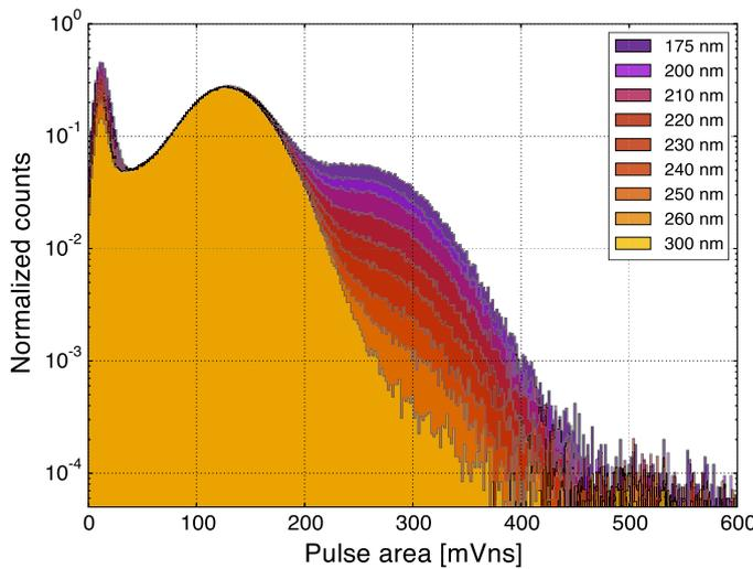
**Figure 16.** Superposition of single photon pulse area spectra of a R11410 PMT for different wavelengths. Each spectrum is normalized by the integral in the region between 50–120 mV ns in order to show the effect more clearly. Reproduced from [500]. © 2015 IOP Publishing Ltd and Sissa Medialab srl. All rights reserved.
