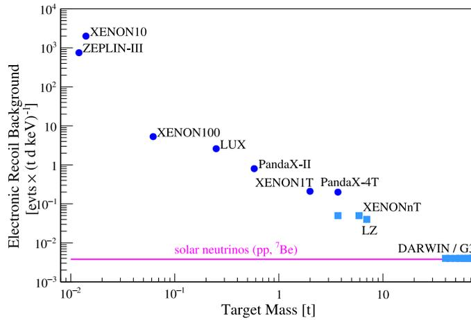
**Figure 3.** The background rates in liquid xenon TPCs (before ER/NR discrimination) have decreased exponentially over the years. This has been a key accomplishment that has enabled an exponential gain in sensitivity with ever-larger detectors. Solid dots are the best achieved limits, open squares the expected sensitivities. The experiment discussed here is labeled DARWIN/G3 and will at low energies be dominated by the signal from solar neutrinos. See text for references.
