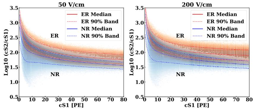
**Figure 37.** Histograms for a flat ER spectrum and a NR spectrum as from a 50 GeV spin-independent WIMP, simulated for different electric fields (using NEST 2.3.5). The top band for each plot is the ER band, the bottom is the NR band. Red lines refer to the median for either band, and the white dotted lines delimit the one-sigma region. Already-demonstrated ER/NR discrimination is expected to be sufficient for a next-generation detector.
