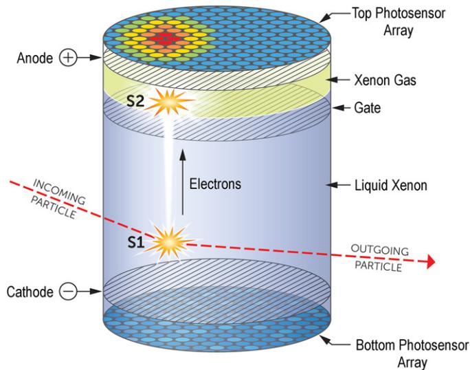
**Figure 4.** Principle of a dual-phase liquid xenon TPC. Energy from a particle interaction within the active liquid xenon volume produces prompt scintillation light (S1) and a delayed signal (S2) from electroluminescence (proportional scintillation) in the gaseous xenon layer. The localization of the S2 signal and the time difference between S1 and S2 allows for determination of the original vertex location.
