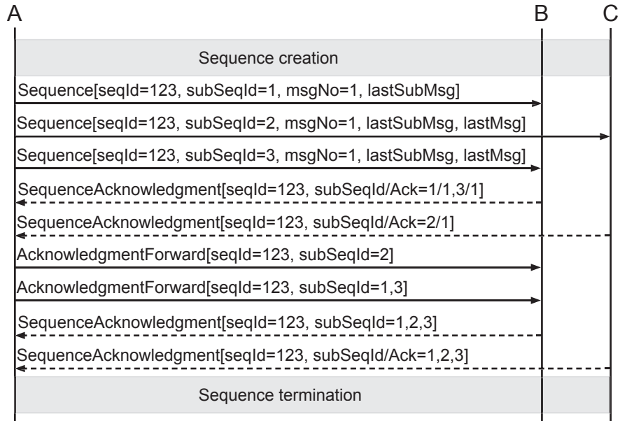
Figure 7.8: The entirely new reliable messaging protocol (non-blocking)
