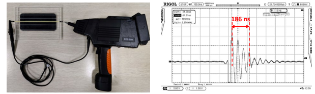
Figure 4: (a) The experiment setup of the feasibility study and (b) a pulse signal generated by the electrostatic gun. The pulse lasts for 186 ns.
