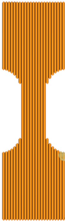
Figure 4.2.: Test geometry with a layer orientation of 0°.
