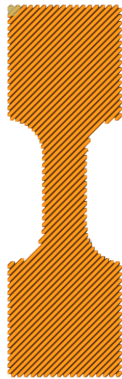
Figure 4.4.: Test geometry with a layer orientation of 45°.
