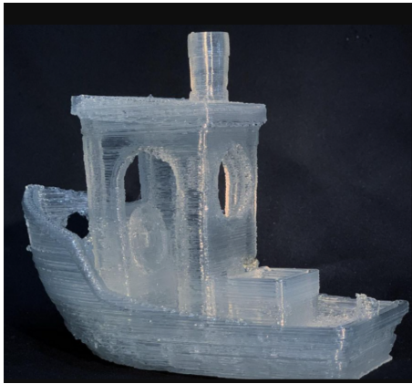
(a) A "benchy" printed by Maple Glass Ltd. with 1 mm layer height [2].
