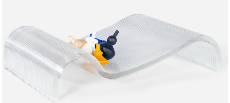
(b) A "wave" printed by Evenline with approx. 5 mm layer height [52].
