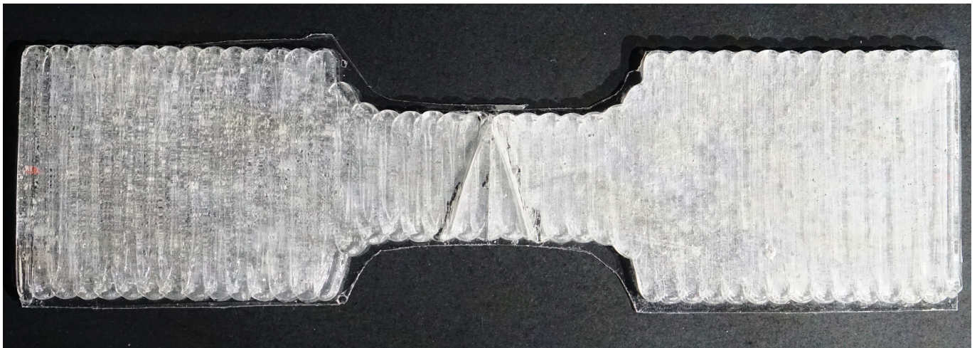
Figure 4.17.: Specimen 90-1 in the fractured state. The specimen is broken into 4 pieces from one fracture origin.
