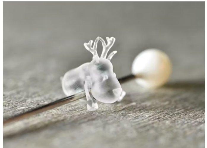
Figure 1.3.: A reindeer made of silica glass using SLE, as big as a pinhead. Moveable legs and head. Produced by the company lightfab GmbH [21]
