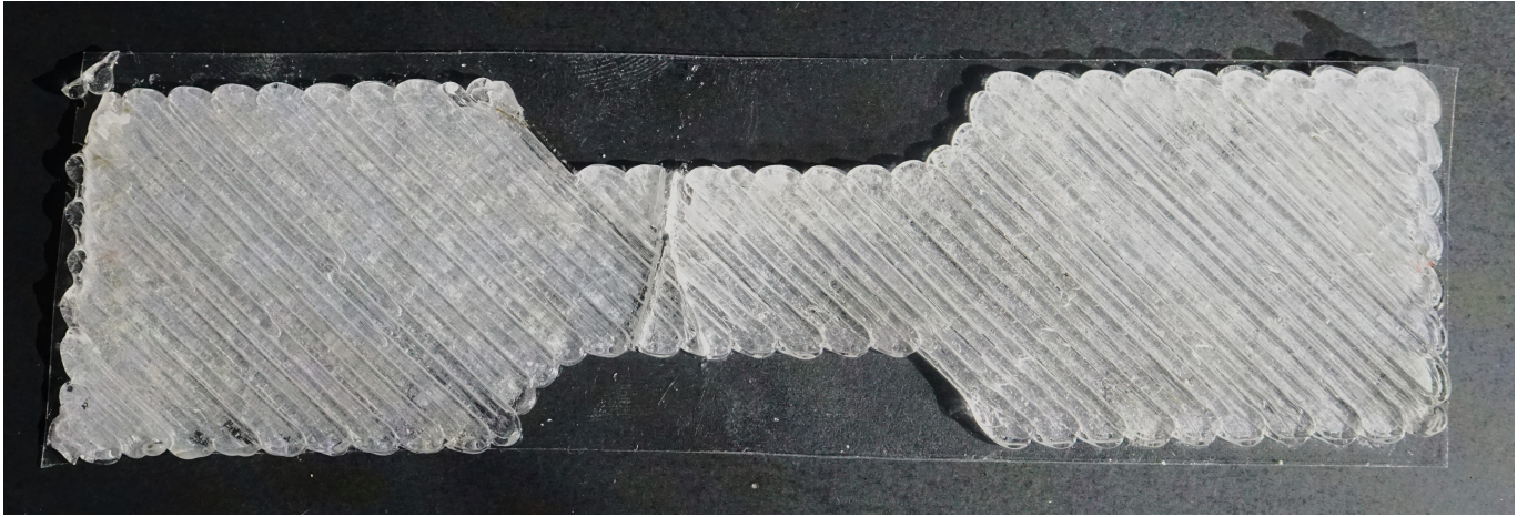
Figure 4.18.: Specimen 45-2 in the fractured state. The crack runs perpendicular to the longitudinal axis of the specimen and then splits into 2 angled cracks.
