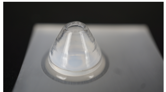
Figure 1.7.: 3d-printed cone made of silica glass with DED from the LZH.
