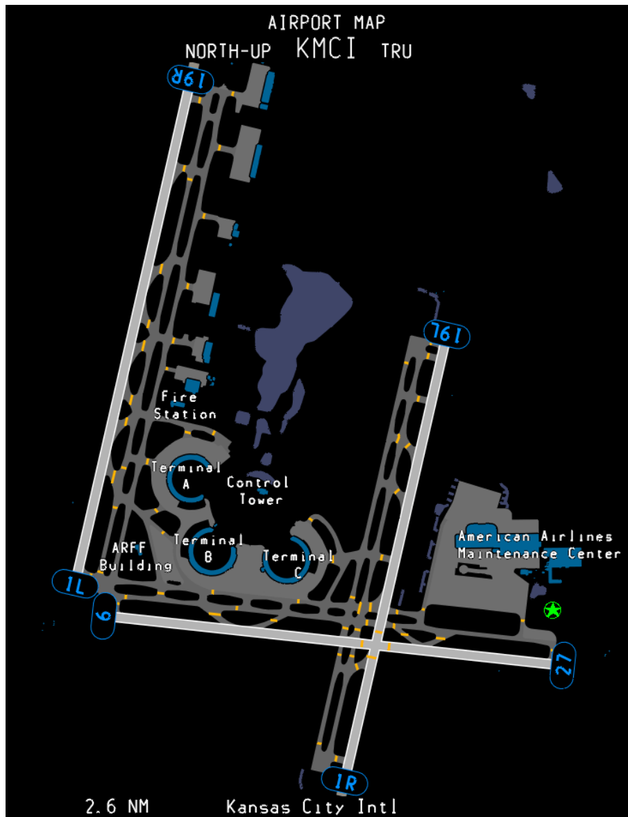
Figure B.4: Building Labels at Kansas City at the 'all airport' zoom level. Only important buildings like the tower and two fire station, the terminals, and the largest cargo hangars are marked.
