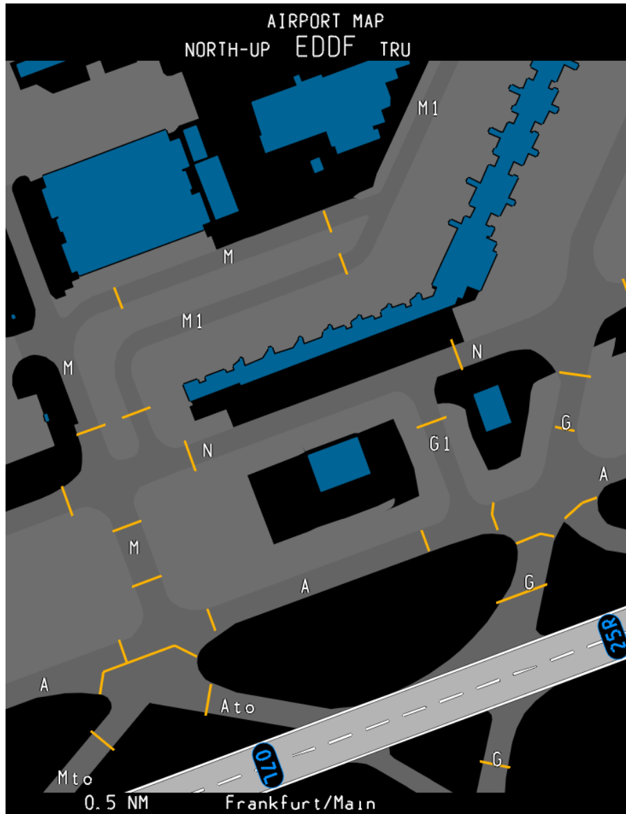
Figure B.10: Taxiway Labels at Frankfurt/Main at the 0.5nm zoom level. No significant changes occur when switching to this zoom range. Most taxiway labels are located completely within their taxiway geometry, minimizing conflicts with parking labels which are normally also displayed at this zoom level.
