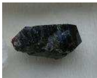
Figure 8.1. – Photograph of a cleaved naturally grown anatase single crystal as used in this work. Facing the camera is the (101) surface plane
