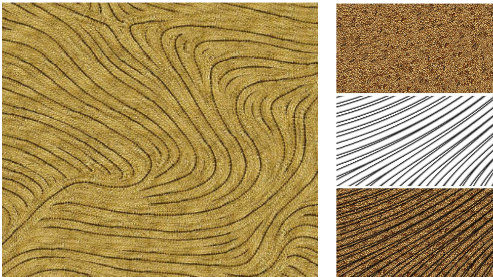
Figure 5.12: Left: using texture-mapped thick streamlines to visualize a flow field. Right: an illustration of texture outlining used to disambiguate streamline orientation.
