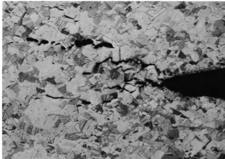
Figure 6: Creep damage in copper at 250°C [1].
