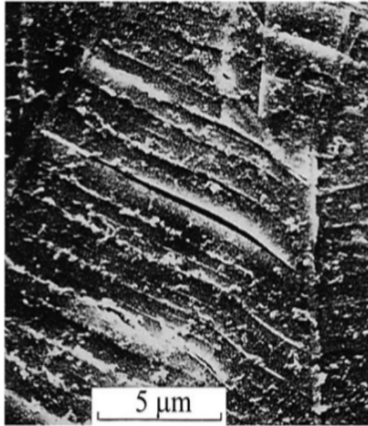
Figure 7: Low cycle fatigue due to glide plane decohesion in Inconel 718 [1].
