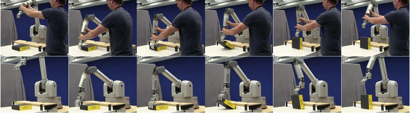
**Figure 3.5.:** Illustration of teaching and reproduction of the box flipping task. The task was to initially move the end-effector to a position close to the box. Subsequently, the box was pushed against the obstacle. Then, the box was flipped. Finally, the end-effector was moved to its final position.
