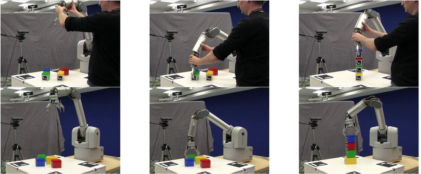
**Figure 3.8.:** Experimental setup for the box stacking task (top) and pictures from the reproduction (bottom). The four boxes were put to random initial positions for each demonstration and the reproduction. They were tracked using AR markers.
