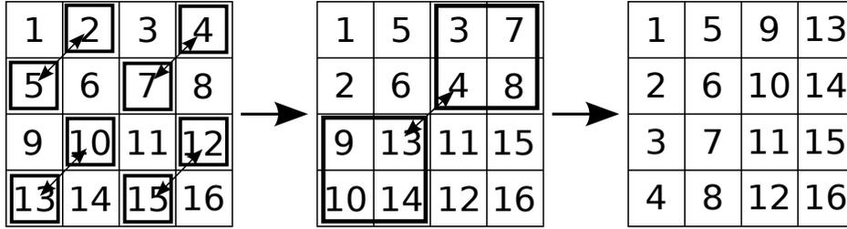
Figure 3.1: Efficient matrix transposition of a  $4 \times 4$  matrix using Eklundh's algorithm.
