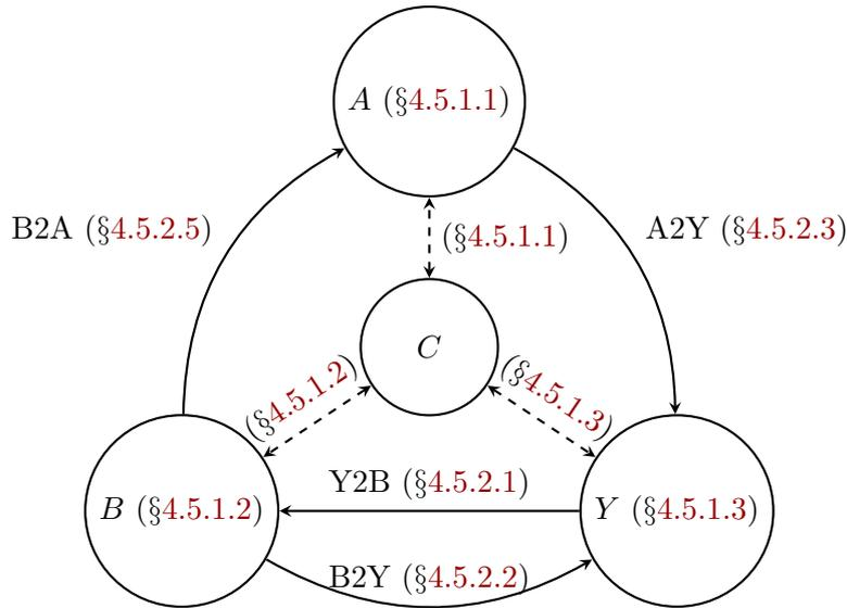
Figure 4.7: Overview of our ABY framework that allows efficient conversions between Cleartext values and secure computation protocols that use **A**rithmetic or **B**oolean secret-sharing or **Y**ao’s garbled circuits.
