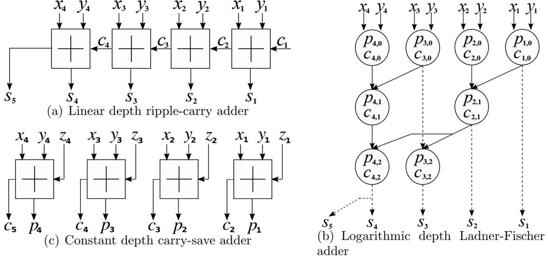
Figure 4.2: Size - and depth efficient addition circuits for two (three) four-bit values.
