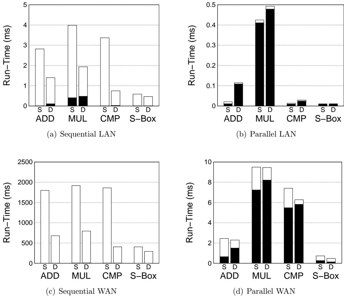
Figure 4.8: Setup time (black) and online time (white) per operation of size (S) and depth (D) efficient circuit constructions (§4.2) using the GMW protocol with 2-MT generation (§4.3.2) in the LAN (a,b) and WAN setting (c,d) amortized over 1 000 sequential operations (a,c) and over 1 000 parallel operations (b,d).
