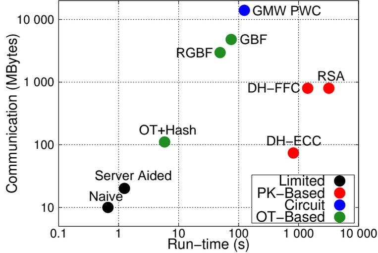
Figure 5.3: LAN run-time in s and communication in MBytes of PSI protocols for  $n_0 = n_1 = 2^{20}$  elements and  $\kappa = 128$ -bit security. Detailed results are given in Table 5.9 and Table 5.11.
