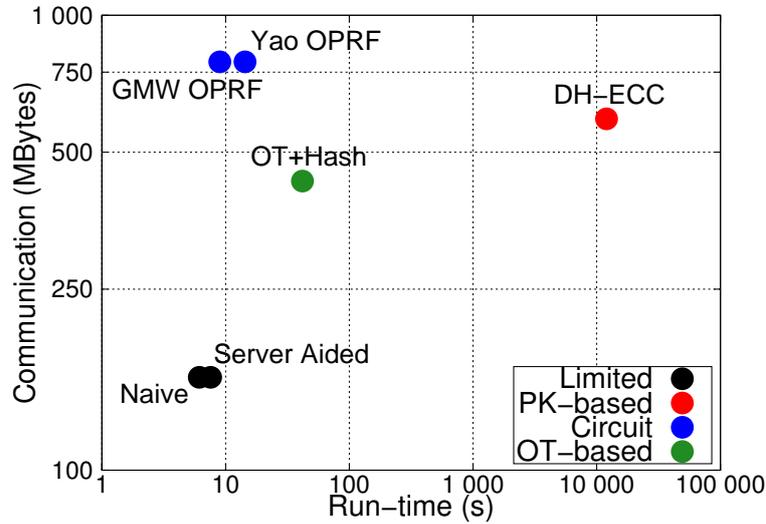
Figure 5.4: LAN run-time in s and communication in MBytes of PSI protocols for unequal sets of  $2^{24} = n_0 \gg n_1 = 2^{12}$  elements and  $\kappa = 128$ -bit security. Detailed results are given in Table 5.13 and Table 5.15.
