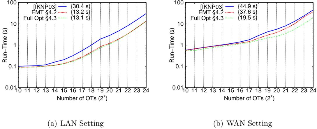
Figure 3.2: Run-time for passive secure R-OT extension on 128-bit strings in the LAN (a) and WAN (b) setting. Time for  $2^{24}$  OTs is given in  $\{\}$ .
