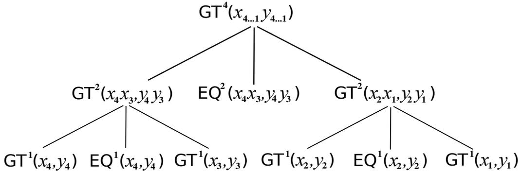
Figure 4.3: Depth-optimized greater than circuit on two 4-bit values.
