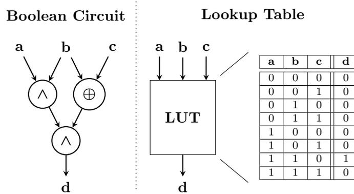
Figure 4.5: A function with  $\ell = 3$  input and  $o = 1$  output bits represented as 2-input Boolean gate circuit and  $(3, 1)$ -LUT.
