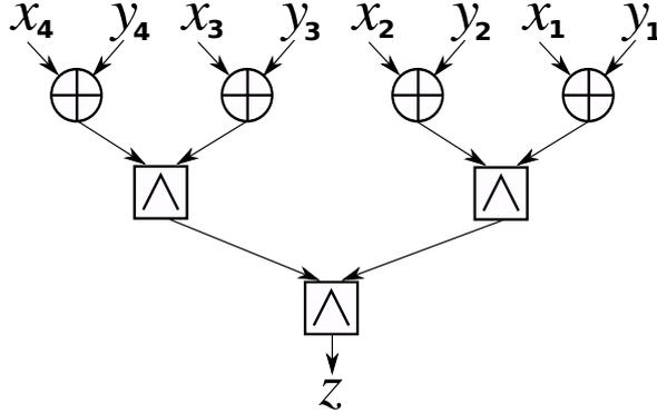
Figure 2.1: Example circuit  $C_{ex}$  with  $\mathbf{S}(C_{ex}) = 3$  and  $\mathbf{D}(C_{ex}) = 2$ .
