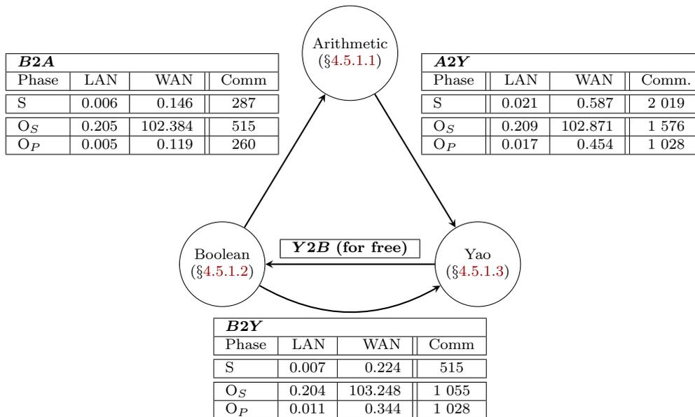
Figure 4.12: Setup (S) and online ( $O_S$ ,  $O_P$ ) time (in *ms*) and communication (in Bytes) for transformations from one share representation to another in the LAN and WAN settings amortized over 1 000 sequential ( $O_S$ ) and 1 000 parallel operations ( $O_P$ ).
