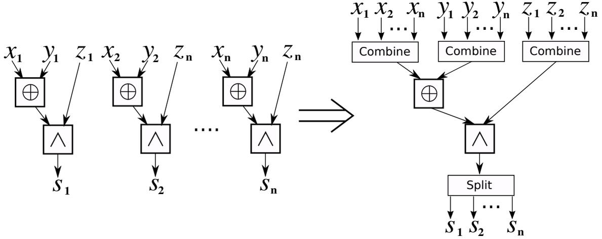
Figure 4.4: One-time evaluation of identical circuits using SIMD operations.
