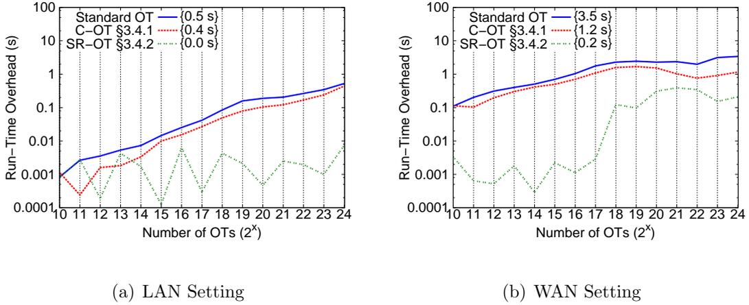
Figure 3.3: Run-time overhead over R-OT for different OT flavors using the semi-honest OT extension on 128-bit strings in the LAN (a)- and WAN (b) setting. Run-time overhead for  $2^{24}$  OTs is given in  $\{\}$ .
