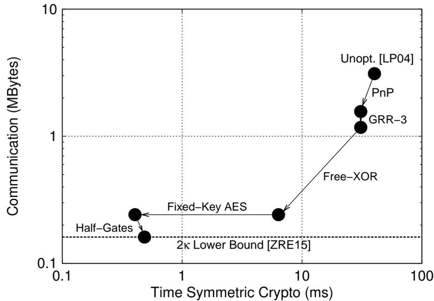
Figure 2.2: Time for symmetric cryptographic operations (x-axis) and communication (y-axis) for different Yao’s garbled circuit optimizations when evaluating the AES circuit of [HEKM11] using the S-Box circuit of [BP10] (24 848 total gates, 5 120 AND gates). Each optimization includes previous optimizations. Time for symmetric crypto was measured using an Intel Haswell i7-4770K CPU with AES-NI support.
