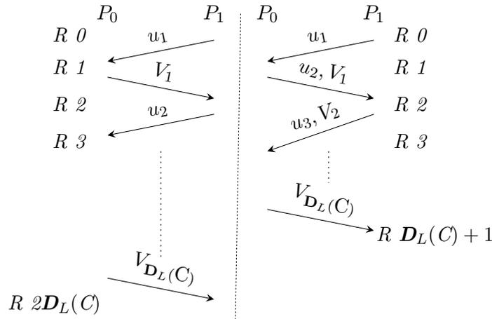
Figure 4.6: Reducing the number of communication rounds for SP-LUT from  $2\mathbf{D}_L(C)$  to  $\mathbf{D}_L(C) + 1$  by flipping roles.
