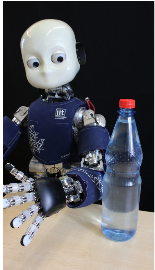
Figure 3.1.: The humanoid robot iCub used in our experiments. The blue artificial skin consists of over 2000 tactile sensors distributed across the whole body.
