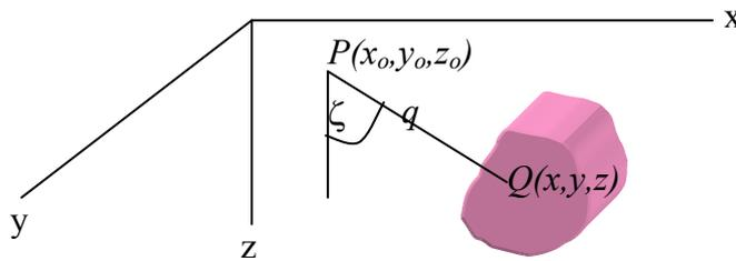
Fig.3.3. Three-dimensional body producing attractions at point P;  $\zeta$  is the angle that the vector  $r$  (from P to Q) makes with the vertical.
