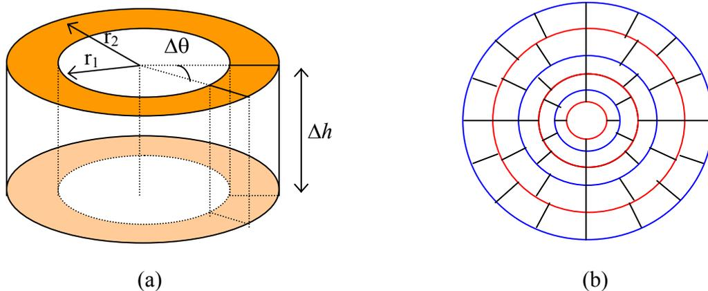
Fig. 3.2a Hollow right-circular cylinder with segments of inner and outer radii  $r_1$  and  $r_2$ , angle  $\Delta\theta$ , and height  $\Delta h$  above (below) station.
