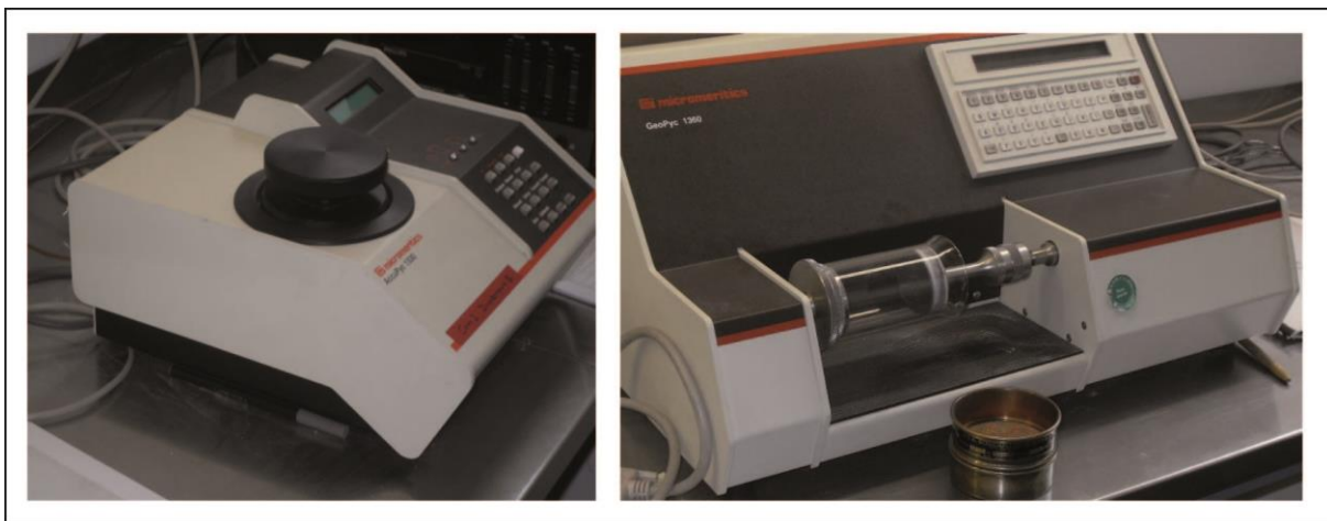
Figure 7: AccupycII 1330 (left) and 1360 (right) Pycnometer at the Institute for Applied Geosciences, Darmstadt.
