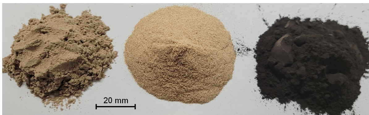
Fig. 6.7 Picture of the three different pulverized fuels (from left to right): beach wood, walnut shells and Rhenish lignite.
