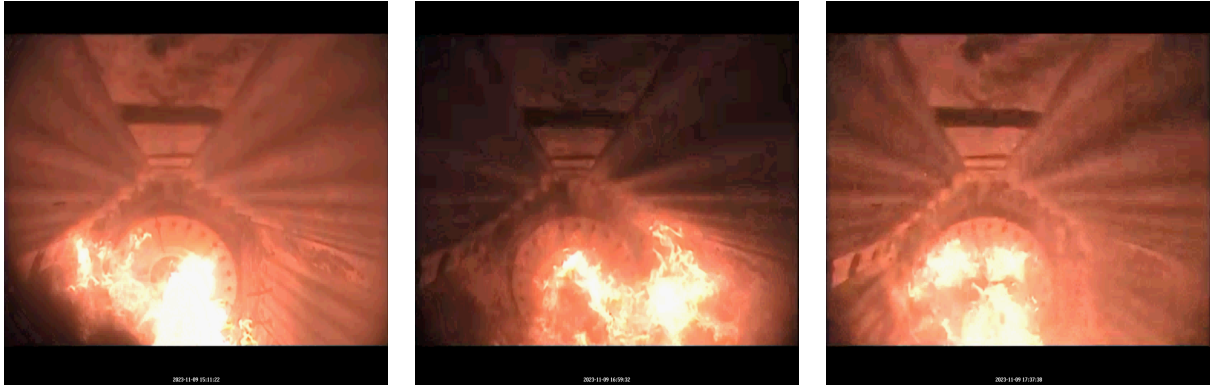
Fig. 7.14 Images of different unstable oxyfuel WS flames. Left: oxyfuel WS flame at 400 kW th with 30 vol% O 2 in the oxidant, \lambda_{loc} = 1.2 . Middle: oxyfuel WS flame at 500 kW th with 26 vol% O 2 in the oxidant, \lambda_{loc} = 1.0 . Right: oxyfuel WS flame at 460 kW th with 33 vol% O 2 in the oxidant, \lambda_{loc} = 0.9 .
