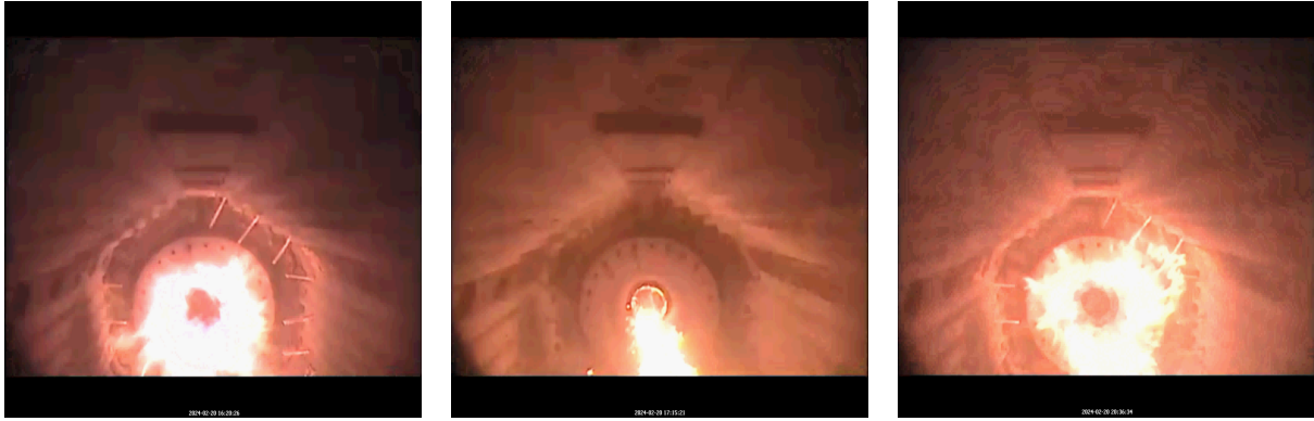
Fig. 7.11 Left: NG flame in air atmosphere (NGAR) with S = 0.96 . Middle: non-swirled NG flame in air atmosphere (NGAR). Right: NG flame in oxyfuel atmosphere with 28 vol% oxygen content in the oxidant and S = 0.93 (NG28).
