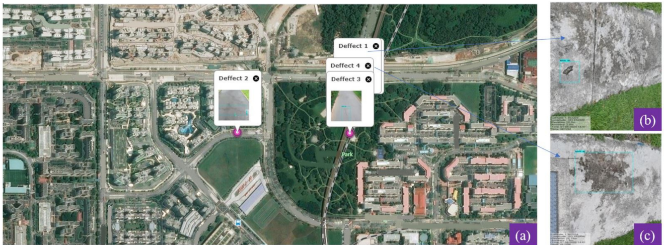
Figure 3-30: Independent trial for the mobile mapping system and the defect identification: (a) Defect location on global map and (b,c) detected defects and patches (Ramalingam et al., 2021)
