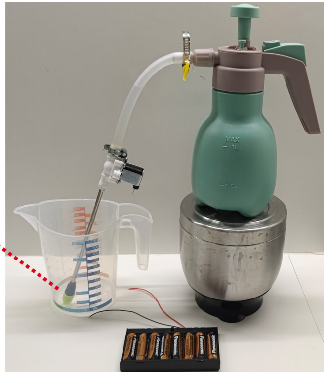
Figure 5-52: Testing the spraying capacity of sprinkler system
