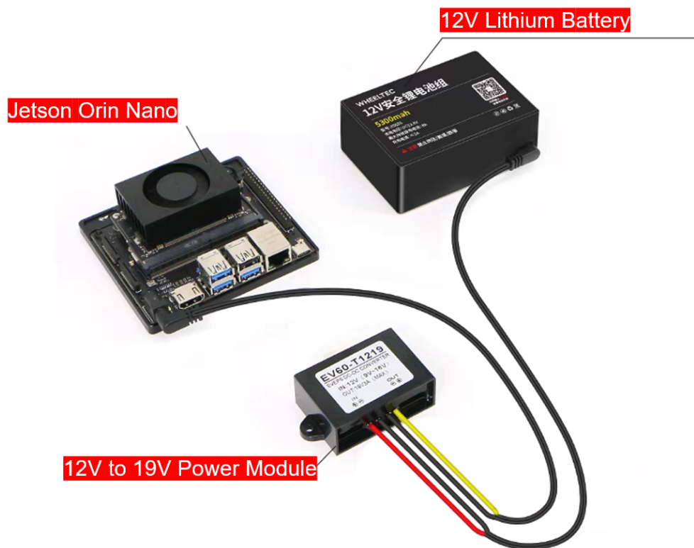
Figure 5-10: Lithium battery and voltage converter for Jetson Orin Nano
