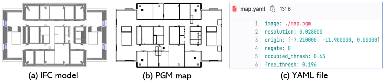
Figure 5-20: Creating PGM map and YAML file from the IFC model of Building L501 of Technical University of Darmstadt
