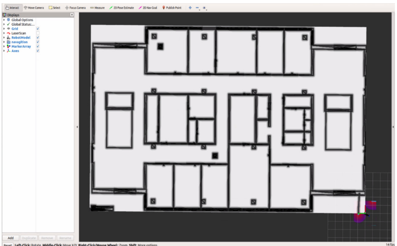
Figure 5-21: Visualization of the PGM map derived from the IFC model in RViz with the origin [0, 0, 0]
