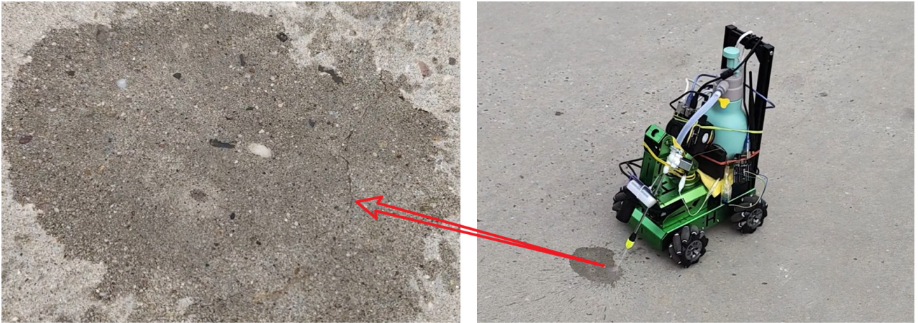
Figure 6-17: Spraying water on narrow cracks upon detection
