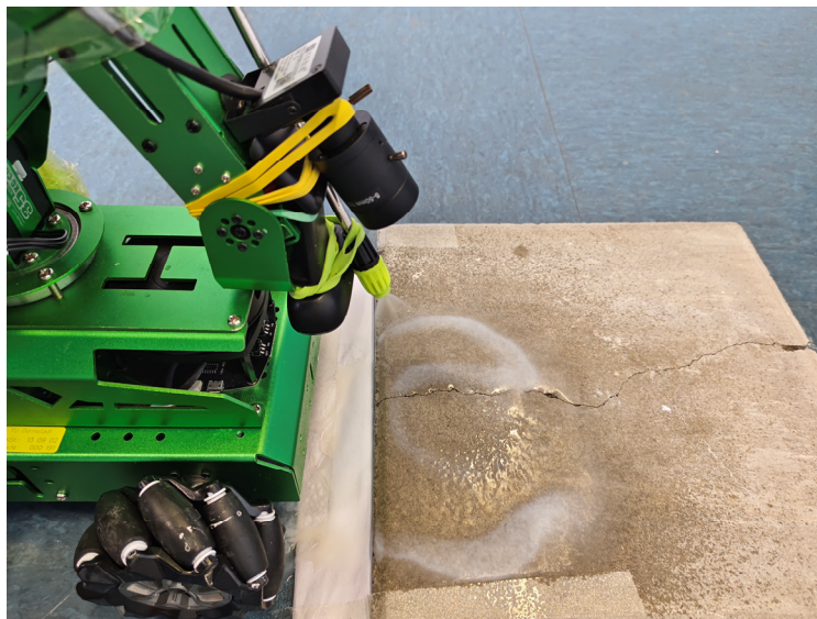
Figure 6-1: Testing robot on concrete slab with narrow crack
