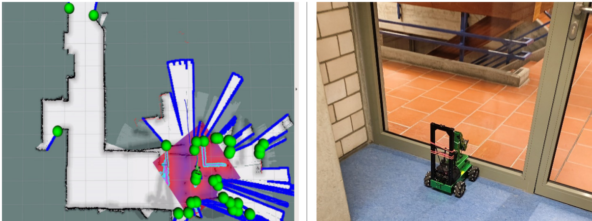
Figure 5-16: Problems encountered when mapping using Explore_lite of JetAuto Pro: bad mapping result (left) and stuck on door (right)
