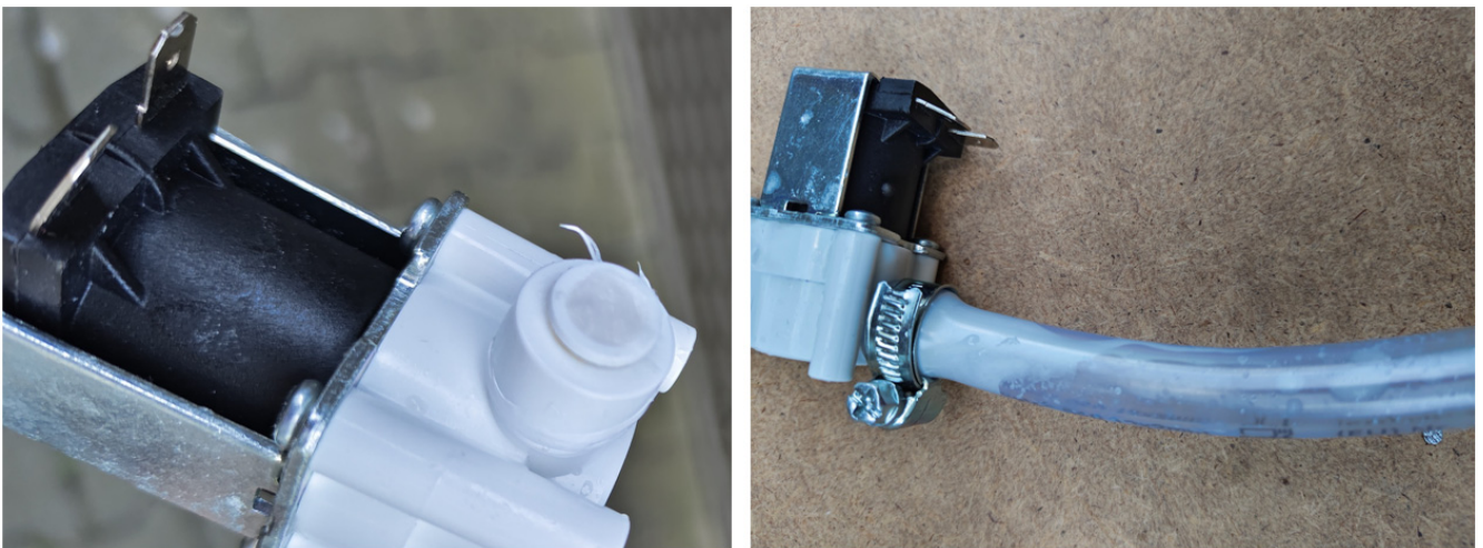
Figure 6-6: Outlet of solenoid water valve clogged by suspension of the solution of component A
