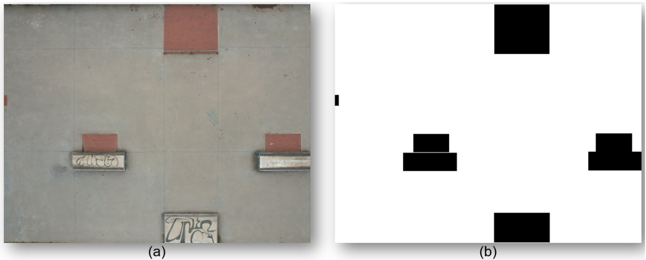
Figure 6-13: Creating map using drone: (a) is aerial image captured by drone and (b) is corresponding PGM map processed by image editor GIMP
