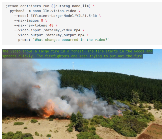
Figure 7-5: Prompt and inference result of live LLaVA-3b model running on Jetson Orin device (NVIDIA, 2024d)
