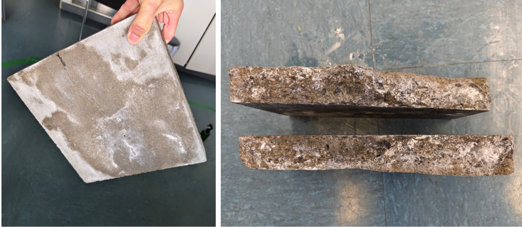
Figure 6-3: Effects of the crack repair after 6 weeks
