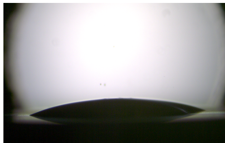
(b) Hydrophilically coated surface, left: sessile droplet after deposition, right: boiling phase exhibiting quiet boiling with only few emerging vapor bubbles
