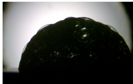
(c) Uncoated surface, left: sessile droplet after deposition, right: boiling phase with considerably increased volume and contact area
