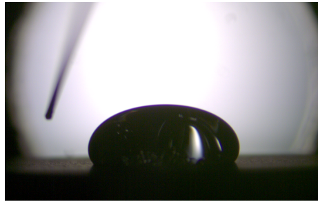
(a) Hydrophobically coated surface, left: sessile droplet after deposition, right: (late) boiling phase
