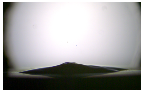
(b) Hydrophilically coated surface, left: sessile droplet after deposition, right: boiling phase exhibiting quiet boiling with only few emerging vapor bubbles
