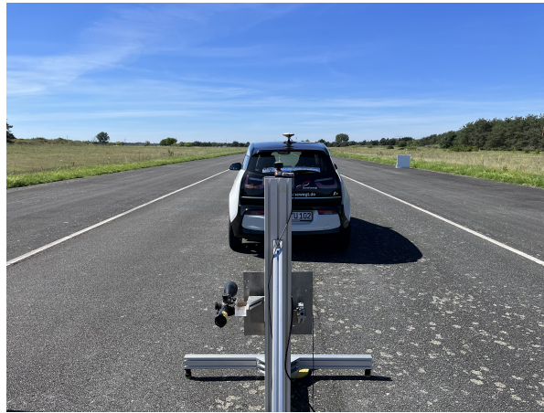
Figure 4-24: Sensor test stand and BMW i3 target vehicle at the beginning of a velocity reference recording.
