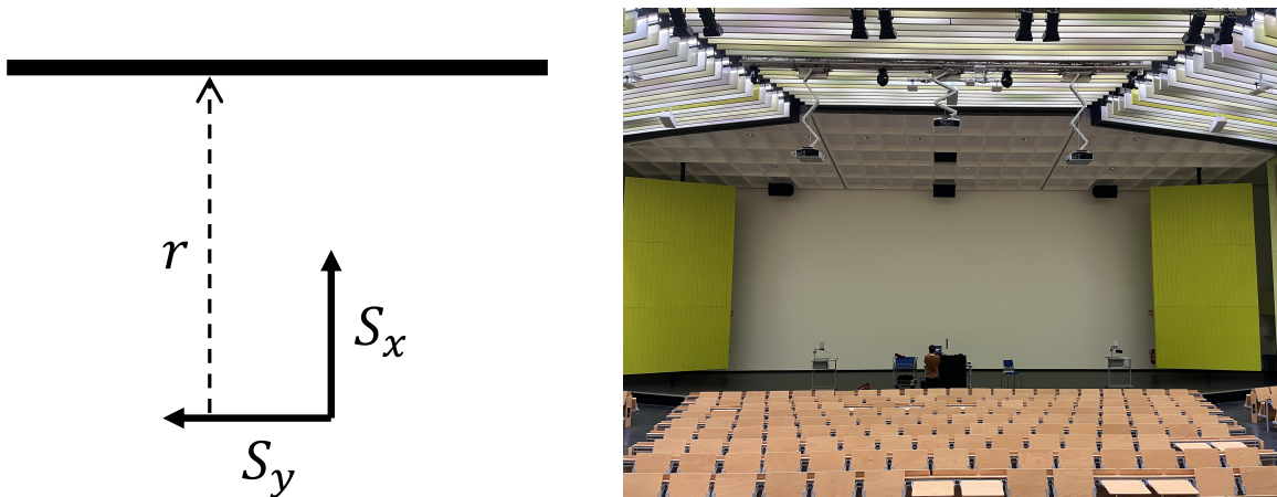
Figure 4-1: The sketch (left) shows the experimental setup of the beam pattern reference measurements. The origin of the coordinate system S indicates the position of the sensor that is placed at a height of 0.749 m above the ground. The range to the wall of the lecture hall (right) is r = 3.056 m.
