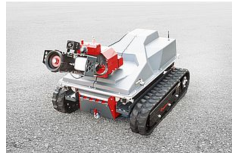
(b) Rosenbauer RTE Robot with a fire fighting monitor (Image: © Rosenbauer International AG)
