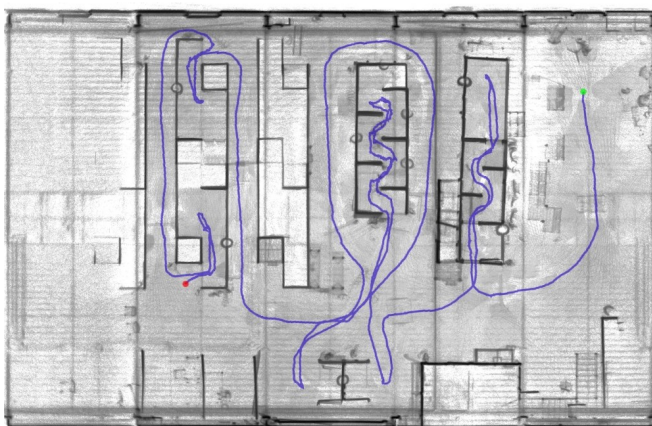
(a) X-Ray of 3D point cloud with the estimated trajectory indicated in blue
