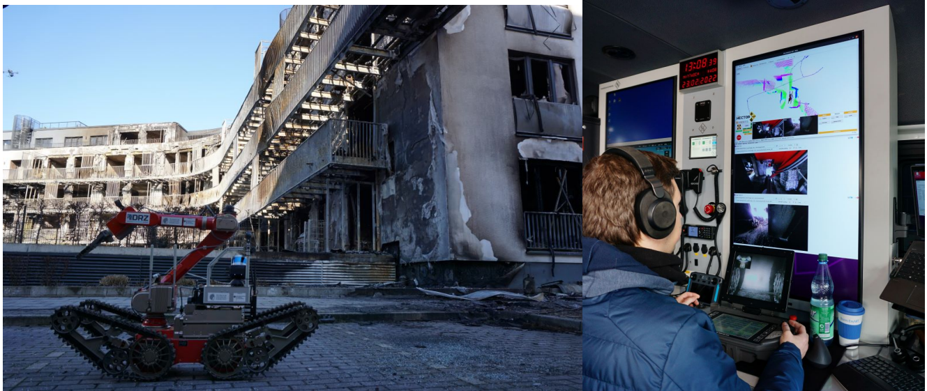
(a) DRZ Telemax robot in front of the building ruins.
