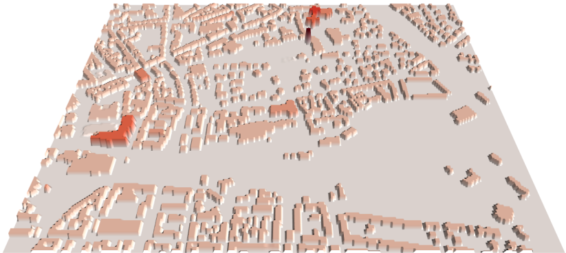
Figure A.3: Height grid map visualization of the Darmstadt map extract derived from OSM data. It contains information on the position of buildings, which is used to derive the risk grid map.
