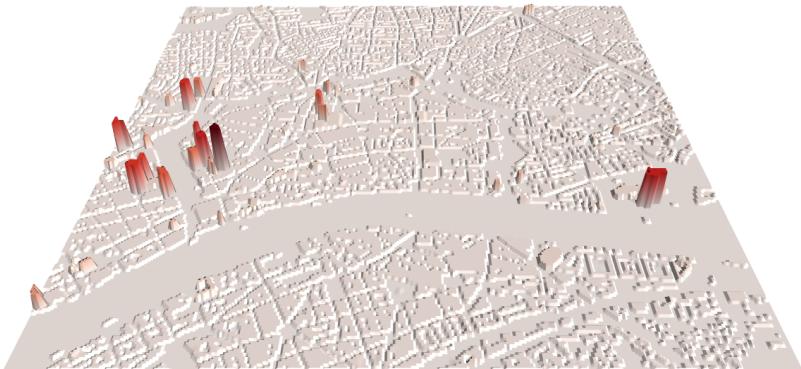
Figure A.21: Height grid map visualization of the Frankfurt map extract derived from OSM data. It contains information on the position of buildings used to derive the risk grid map and the building heights used to calculate the obstacle collision avoidance constraint.
