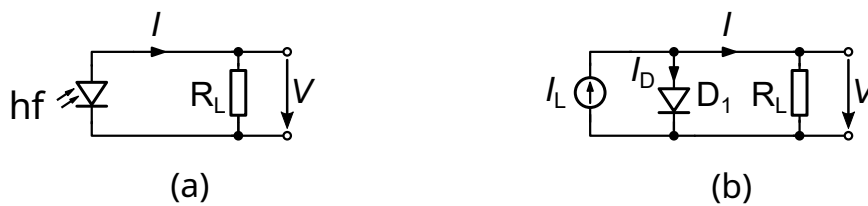
Figure 3.2.: Equivalent circuit for solar cells. Figure (a) shows a solar cell with a connected load resistance, and Figure (b) an equivalent circuit consisting of an ideal current source and a diode substituting the solar cell.
