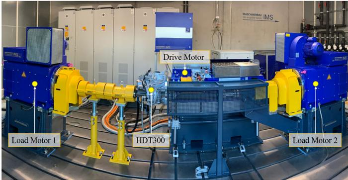
**Figure 1.5:** Test bench for validating Active vibration control using HDT300
