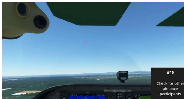
Figure 10: Exemplary MSFS2020 scene with detected aircraft in magenta bounding box (NEEF)
