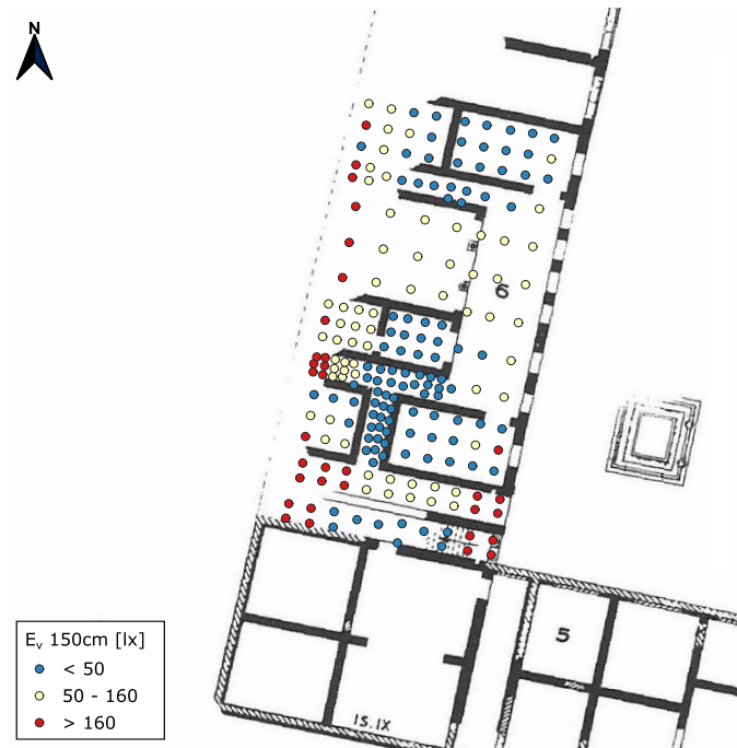
Figure 9. Annual daylight conditions by thresholds for contrast and colour vision on vertical surfaces at 1.50 m height during the first half of the day in the month with lowest daylight admission (basemap by Cervi [12]).
