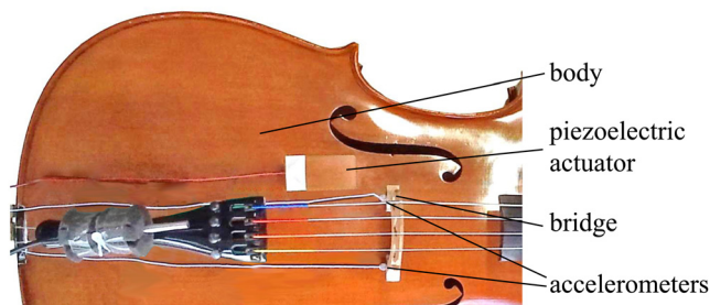
FIG. 12. (Color online) Experimental setup of the validation of the smart materials wolf note eliminator.
