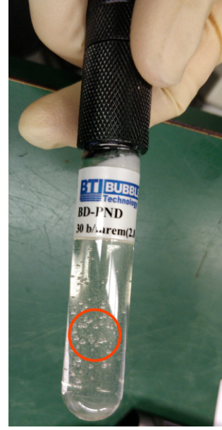
Figure 3.4.: A bubble detector after irradiation. The orange circle contains the detector signal. These are the bubbles indicated by variable b in Equation 3.11.
