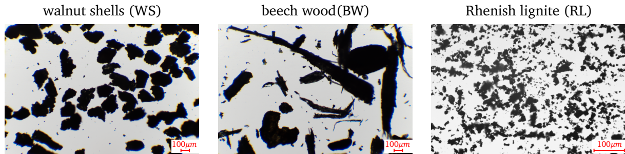
Figure 3.6: Microscopic images of walnut shells (WS), beech wood (BW), and Rhenish lignite (RL). The scale of the images is shown in the lower right corner.
