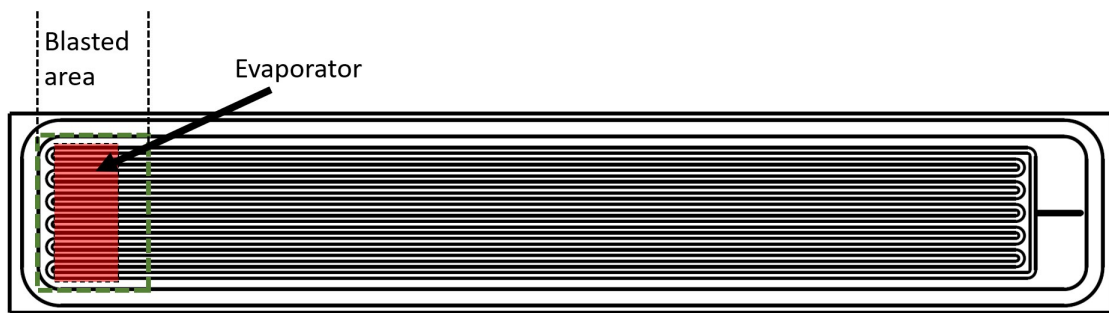
Figure 4.12: Blasted areas of test setups 2 and 3
