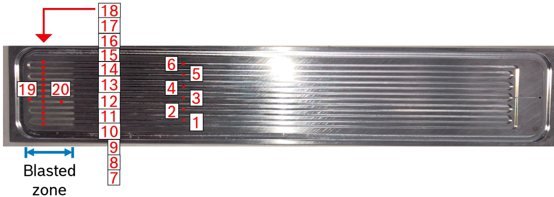
Figure 4.17: Surface measurement positions of test setups 2 and 3
