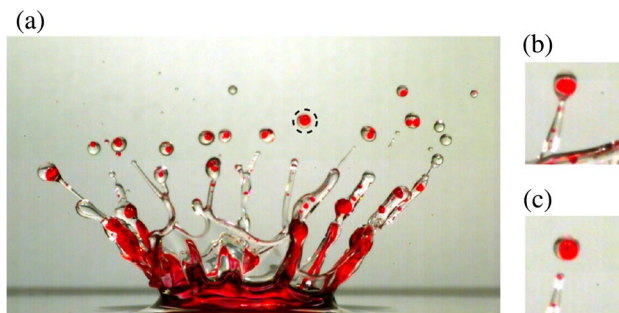
Fig. 1 a Snapshot of a red-colored water droplet ( D = 3 mm, u = 3.2 m/s) impinging onto a film of silicone oil ( \nu = 10 \times 10^{-6} m 2 s -1 ) of 600 \mu m thickness, illustrating the generated secondary droplets; b , c Time sequence of secondary droplets ejected from finger jets
