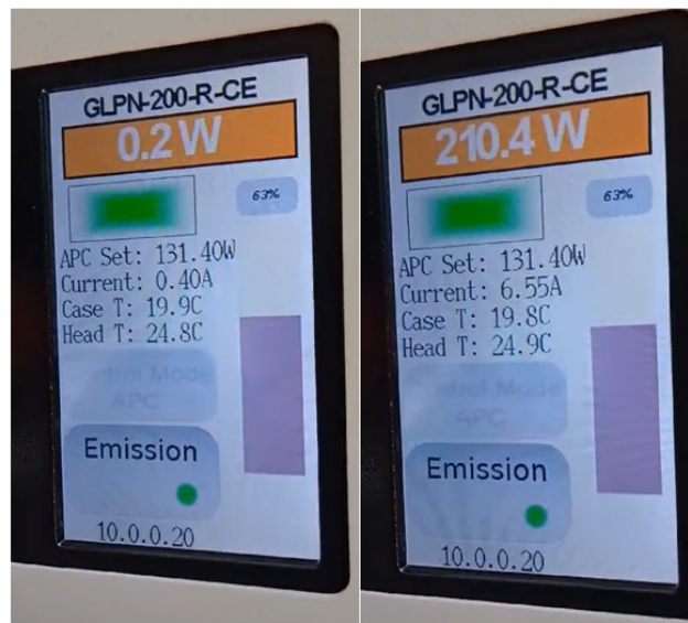
Figure A.1: Laser display showing discrepancies between set and executed laser power
