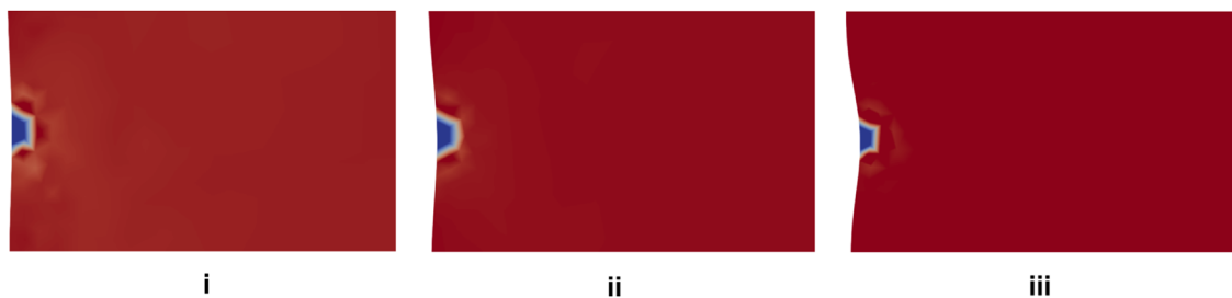
FIGURE 5 The first crack can be found at the same position ( i : scaling with 0.5; ii : original surface profile; iii : scaling with 2) using an example of profile a . Red indicates a crack field variable of s = 1 and blue indicates s = 0 .
