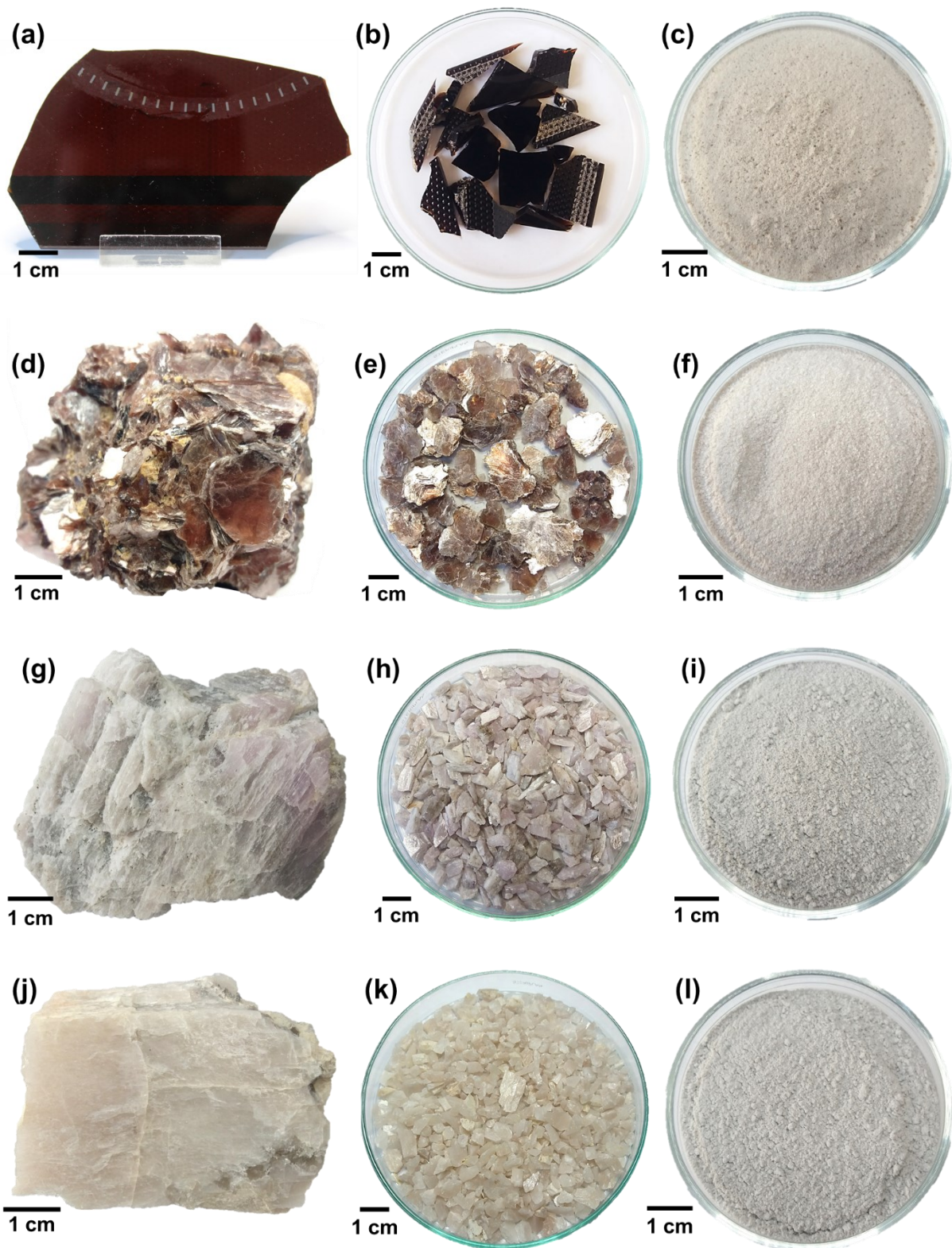
Figure 3-1. (a) to (c) Glass-ceramic samples derived from an end-of-life cooktop, (a) shard after manual dismantling, (b) after jaw crushing and (c) powder < 500 \mu\text{m} . (d) to (f) Lepidolite samples from the Bikita pegmatite, Simbabwe, (d) as received, (e) flakes after jaw crushing and (f) powder < 500 \mu\text{m} . (g) to (i) Spodumene samples from the Sahatany pegmatite, Madagascar, (g) as received, (h) cleavage pieces after jaw crushing and (i) powder < 500 \mu\text{m} . (j) to (l) Petalite samples from the Luolamäki pegmatite, Finland, (j) as received, (k) cleavage pieces after jaw crushing and (l) powder < 500 \mu\text{m} .
