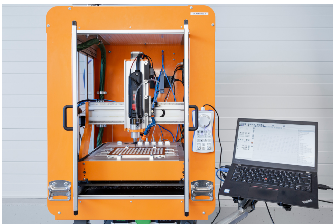
(a) CNC machine used for acquiring the datasets with the attached laptop running the NC control software WINPC-NC.
