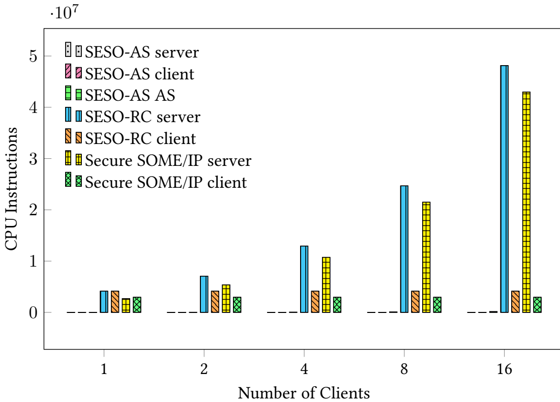
Figure 6.14.: Additional CPU Instructions for Cryptography
