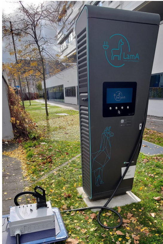
Figure 7.11.: Evaluation Environment for ISO 15118 communication
