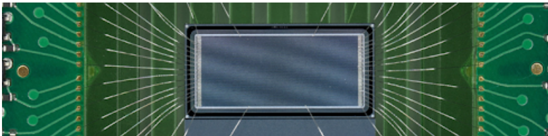
Figure 4.1: Photo of the LGAD sensor mounted on the PCB, used in the first proof-of-principle test at the S-DALINAC. Taken from [50].
