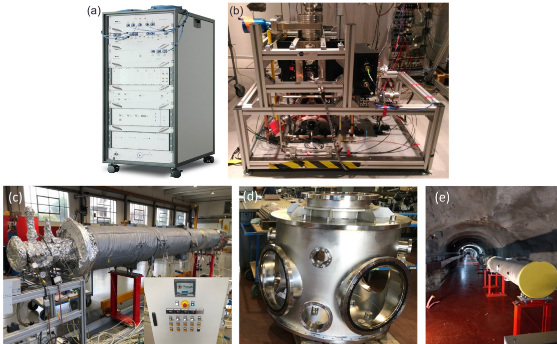
FIG. 20. (a) Fiber laser system developed by the Muquans company, reused with permission from Sabulsky et al. , Sci. Rep. 10 , 021101 (2020). Copyright 2020 Authors, licensed under a Creative Commons Attribution Unported License. 325 (b) cold ^{87}\text{Rb} atom source, reused with permission from Beauflis et al. , Sci. Rep. 12 , 231102 (2022). Copyright 2020 Authors, licensed under a Creative Commons Attribution Unported License. 267 (c) standard 6 m long section under vacuum test, (d) vacuum tower in production at SAES Parma (Italy), (e) MIGA gallery within the Laboratoire Souterrain à Bas Bruit (LSBB) and installation of the first sections of the vacuum vessel, reproduced with permission from Canuel et al. , “A gravity antenna based on quantum technologies: MIGA,” arXiv:2204.12137. Copyright 2022. 326
