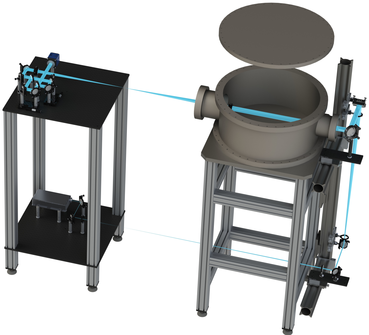
Figure 3.13: Overview of the designed system. The experimental setup consists of two base frames: one supporting the Z4 target chamber and the other holding two breadboards on different levels. The laser frontend is located on the lower level, with its beam directed by two mirrors toward an enlarging telescope. The first lens of the telescope is positioned on the breadboard, and the second lens is placed on a rail attached to the base frame of the target chamber. A mirror behind the second lens directs the horizontal beam to a magnifying telescope, which utilizes a vertical structural rail for its lenses. The beam is finally directed into the Z4 target chamber by a tilting mirror. Within the chamber, the beam fully surrounds the plasma at its center. The beam passes through the first doublet of a telescope, with the second doublet positioned on the upper breadboard. This telescope reduces the beam diameter and images the plasma on the camera. The camera is situated behind a Mach-Zehnder interferometer on the upper level of the optical table. The displayed laser beam diameter corresponds to its actual size. The graphic is taken from Grimm 2023.
