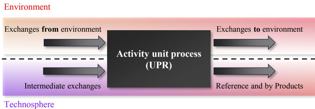
Figure 2.4: Unit process definition
