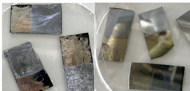
Figure 5.4: Samples of EC (left) and DMO (right) on Si-wafers. Half of the sample was sputtered with 20 nm of gold to obtain a reflecting surface for the measuring of the height via white light interferometry. The ellipsometry measurements were carried out on the non-sputtered part of the sample ( \lambda (laser) = 658 nm; RT; 15 % rel. H.; e34).
