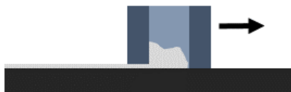
Figure 4.6: Mechanism of coating a substrate with a film frame applicator. The coating solution is placed inside the frame and dragged over the substrate.
