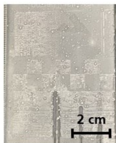
Figure 6.42: Test print of a sample with 31 % urea in PVA with a standard thermoprinter.
