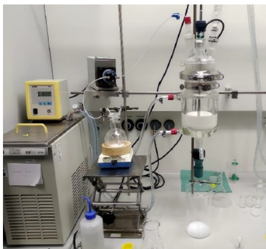
Figure 8.1: Experimental setup of the starved feed emulsion polymerization.
