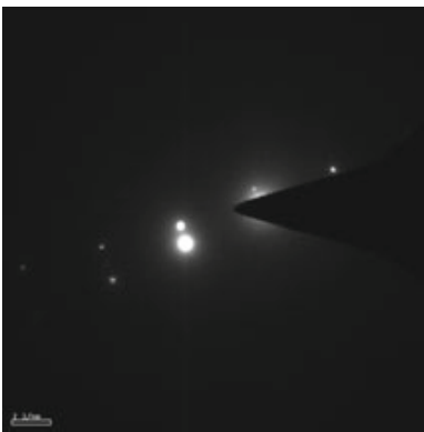
Figure 11-36: A randomly aligned crystal results in an asymmetric diffraction pattern with no relation among diffraction spots. Reprinted with permission from [98], © 2022 Springer Nature Singapore.
