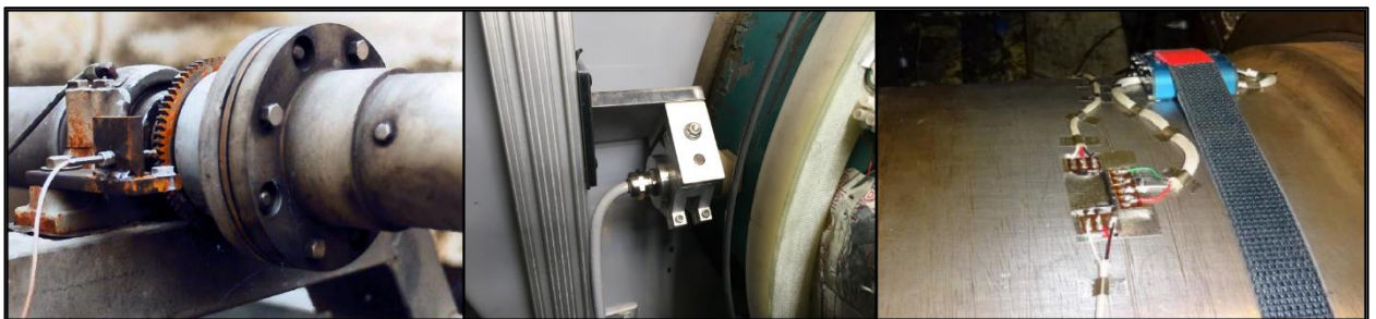
Figure 2 – Eddy-current sensor viewing a toothed wheel (left pane), magnetostrictive sensor viewing a shaft (middle pane), and a strain gage mounted to a shaft (right pane).
